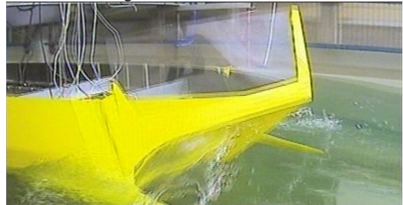
h- Bow comes up further, the water splash extends forward
