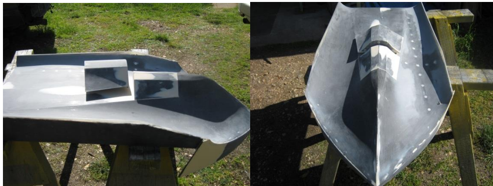
Figure 3.8: Three centrebow length segments under construction. The short centrebow achieved by cutting 150mm from centrebow aft and a separate segment was built to form the long centrebow
