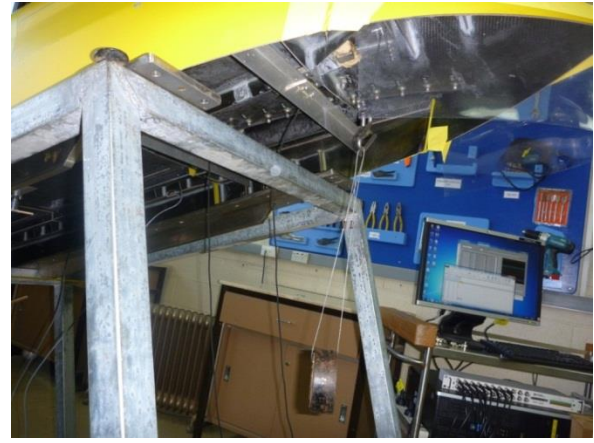
(b)The weights were hung with ahook and string from the centrebow
