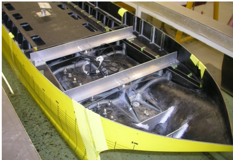
Figure 3.30: The centrebow with pressure transducer casings installed after construction
