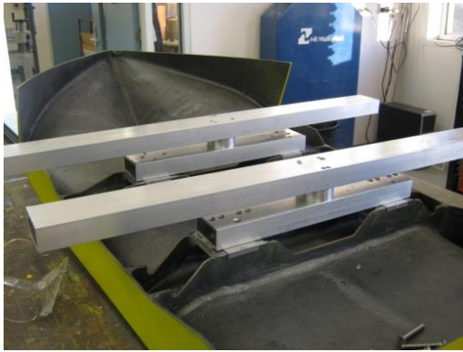
Figure 0.4: Aluminium blocks and the holding frames of the mock up centrebow load measuring system
