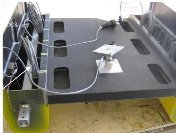
Figure 3.14: HSM02 mid segment wetdeck and demihulls assembly configuration
