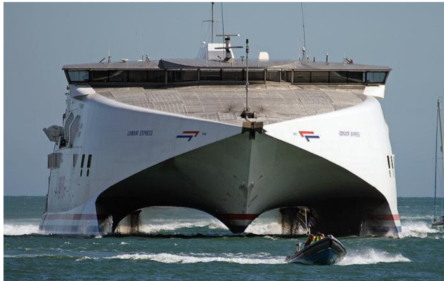
Figure 1.3: Condor Express, INCAT Hull042, an 86m car-passenger wave piercing catamaran (Barry Quince). The centrebow can be seen between the two demihulls
