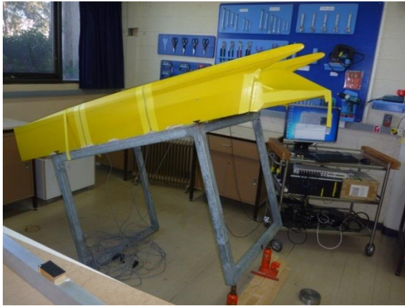
(a)The model set up in 19.7 degree Position for loading the centrebow
