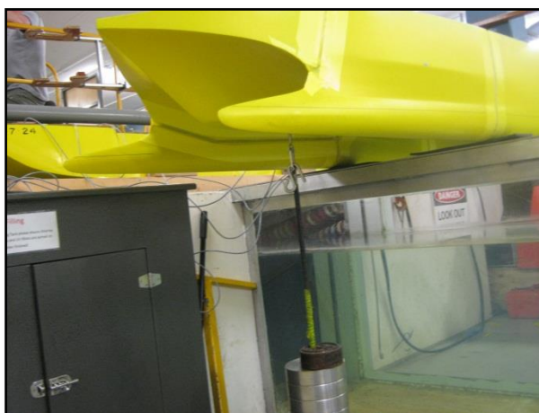
(a) Loading the model for Forward cut VBM calibration in Position 2
