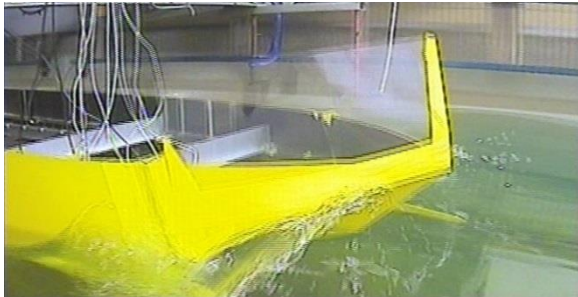
g- Water starts splashes outboard, bow up motion starts
