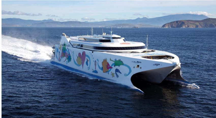
Figure 2.4: Natchan Rera, INCAT 112 m wave-piercing catamaran ( www.INCAT.com.au ) showing the fine entry demihull bows and the centrebow
