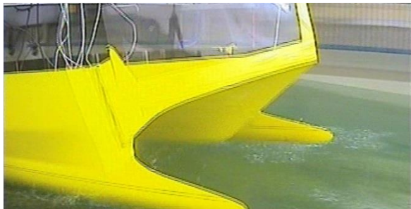
j- Both the centrebow and demihull bows emerge from water again
