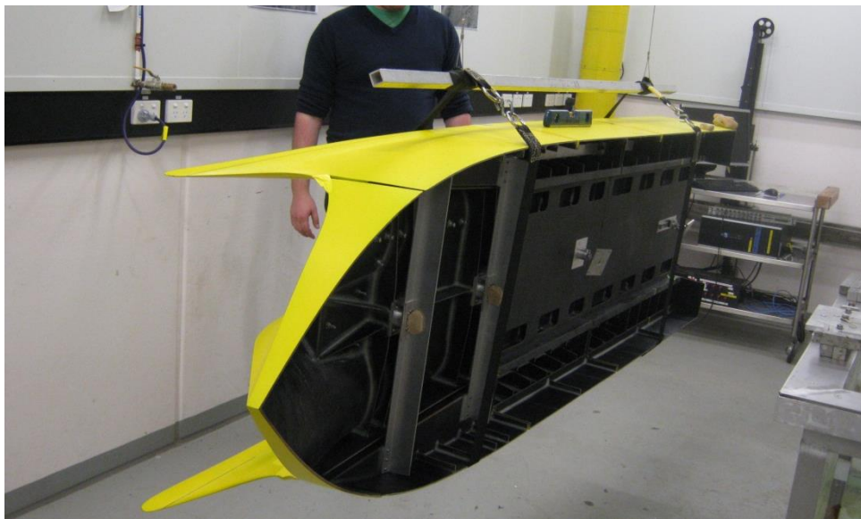
Figure 5.2: The set up for Bifilar swing test to estimate the model pitch radius of gyration
