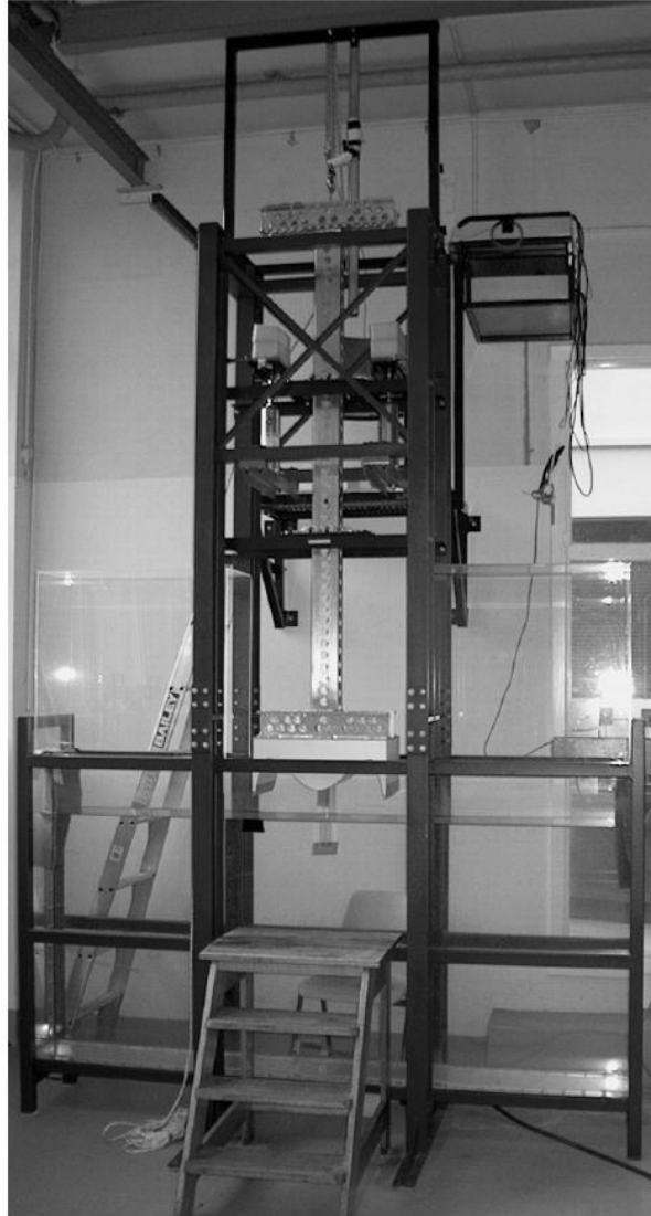
Figure 1.4: The drop test rig of Whelan in University of Tasmania [12, 33]. Catamaran sections with centrebows were free dropped into water tank
