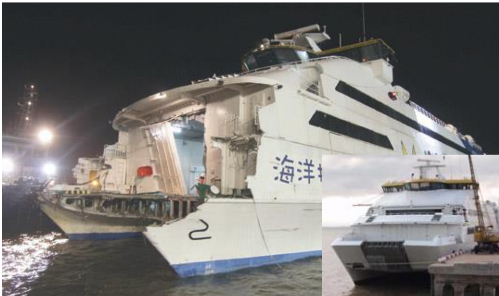
Figure 1.2: Ocean Lala, the catamaran ferry losing the bow structure from severe wetdeck slamming in Taiwan waters. The waves have damaged the front car ramp, cross deck structure, front bulkhead and gate. The lower right: the vessel before damage occurred ( http://www.chinapost.com.tw , http://www.gov.cn/english/2009-07/16/content_1366854.htm )
