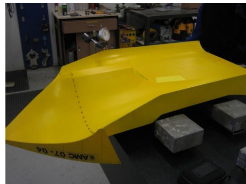
Figure 0.5: Measuring the deflection of the centrebow edge under asymmetric loading with a dial gauge. The centrebow was fixed upside down on aluminium frames.
