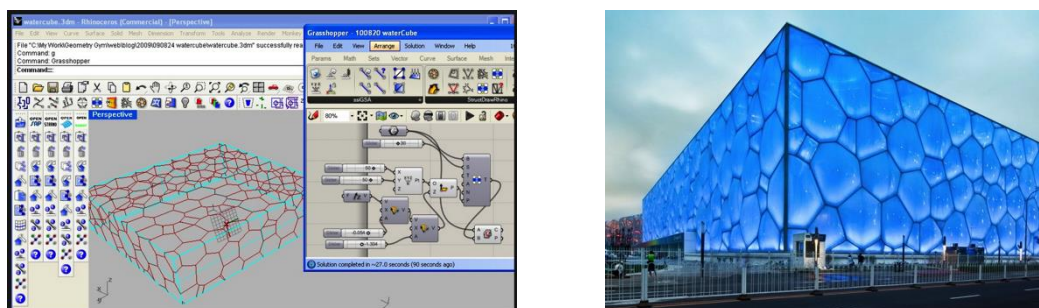
Figure 26 The Rhino and Grasshopper software were used to demonstrate the ‘coded’ modelling of a 3D tessellation, which was completed just in 27 seconds. The Beijing Watercube Olympic swimming stadium is an example using this geometry.
