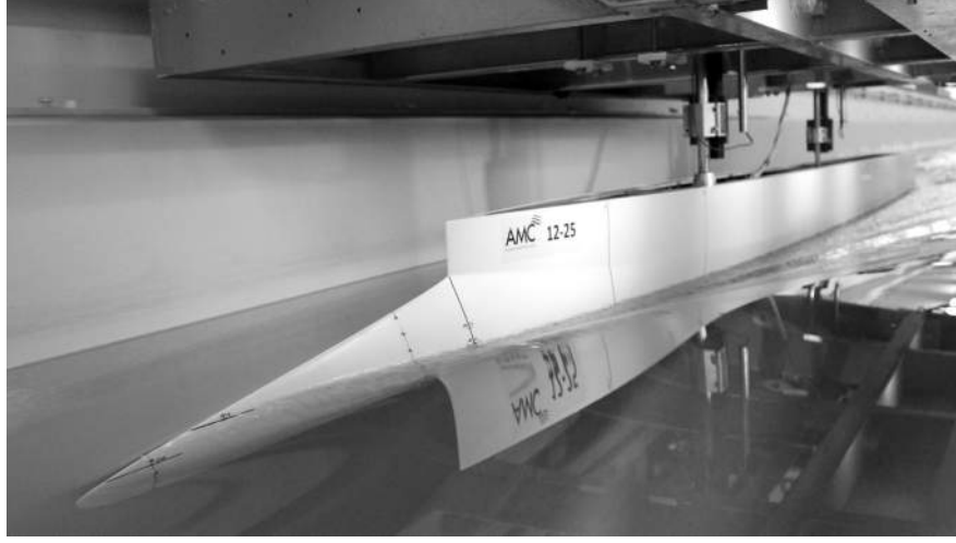
Figure 3.5: Half model of the 98 m catamaran as it was tested in the AMC towing tank.
