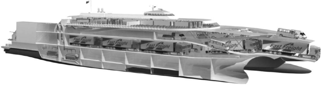
Figure 1.2: Arrangement of a large medium-speed catamaran proposed by Davidson et al. (2011b).
