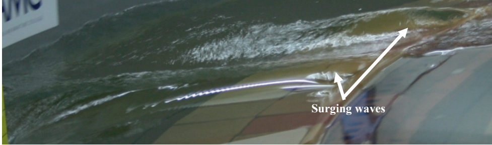
Figure 2-8. Surging waves generated by condition 50 model 12-02 with \xi = 3.3 , d^* = 0.2 in h_0 = 250\text{mm} at Fr_{h0} = 0.9 , s = 23^\circ and y_{beach}^* = 1.4 .
