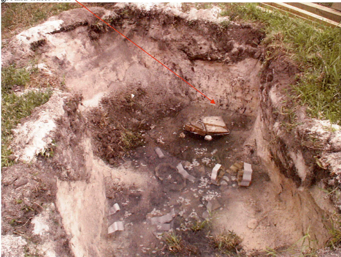
Figure 4.4 Test hole showing ground water at approximately 1m ground water level
