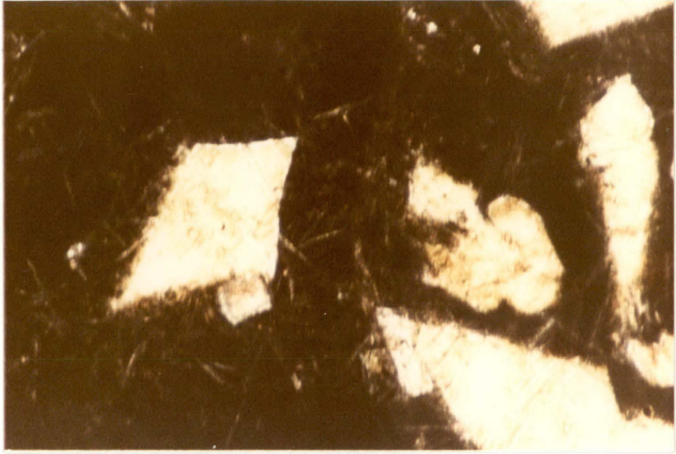
Figure 3.5. Photomicrograph of the studied ocean-island tholeiitic lava (Subgroup A-1)(sample 56.3) showing altered olivine microphenocrysts and glassy groundmass made up largely of dark brown glass, and stellate and variolitic aggregates of quenched plagioclase crystals. Ordinary light, X 65.
