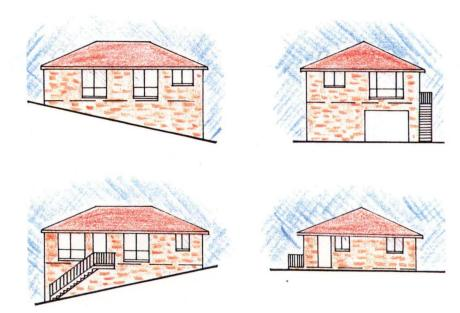
Figure 39: Design "Solution" for a Sloping Block - An Excavator, Plenty of Bricks and a Set of Steps!
