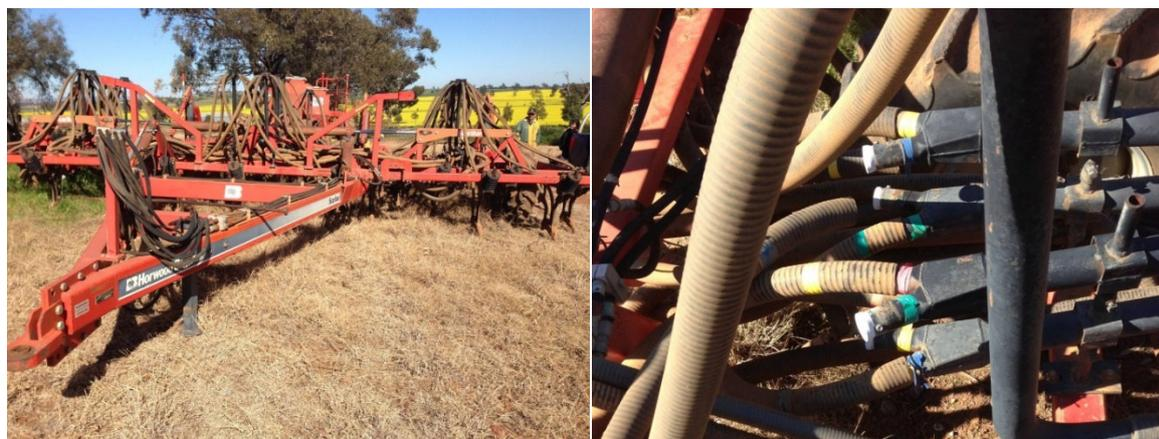
**Fig. 1.** An example of a commercial seeder ordinarily used by a local Wagga Wagga grower to sow pasture components in alternate drill rows. Right: Flows to specific tynes can be blocked allowing different species to flow to separate tynes. In this example, lucerne was delivered from the fertilizer box while phalaris was delivered from the seed box.
