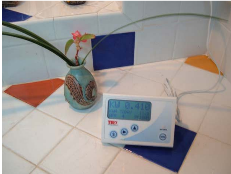
Figure 12. The Energy Detective (TED) in-home display (Parker et al. 2008).
