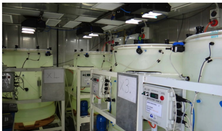
Figure 2.1: Minicosm tanks filled with seawater in temperature-controlled shipping container.
