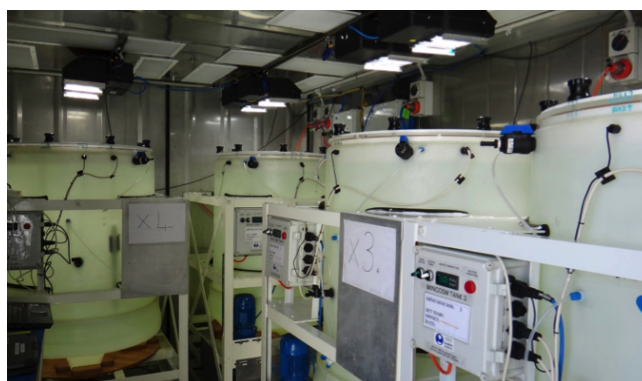
Figure 1. Minicosm tanks filled with seawater in a temperature-controlled shipping container.
