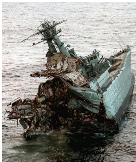
Figure 1-12 Bubble jet damage from a heavy weight torpedo detonation under the amidships section of the decommissioned HMAS Torrens [26]
