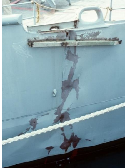
Figure 1-13 Buckling damage to the hull plate from UNDEX induced whipping due to a mine strike on USS Princeton (CG-59) [29]
