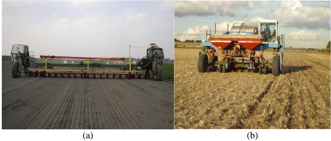
Figure 6-4. Attempts at commercialisation of wide span gantries in the 1980-90s included (a) the Dowler gantry and (b) the Ashot Ashkelon Industries Ltd Field Power Unit (FPU). (Source: W.C.T. Chamen)
