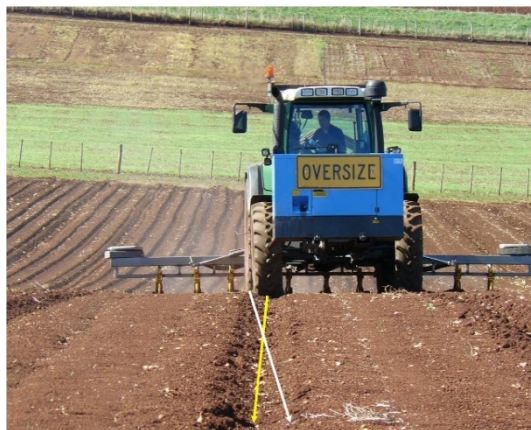
Figure 3-3. Sideways slip of tractor on compacted controlled traffic wheel tracks during fertiliser pre-drilling (left) and a non-draft operation, mulching (right).
