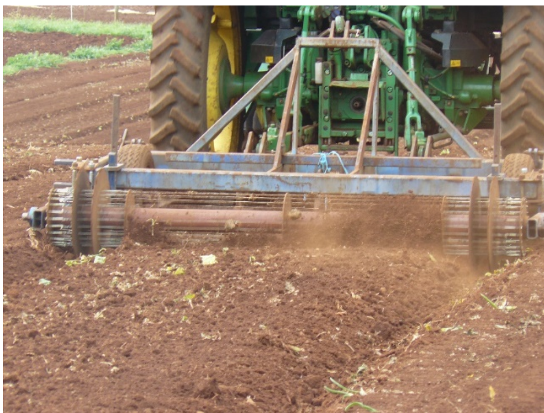
Figure 3-1. Wire roller used after ripping to provide final seedbed condition.
