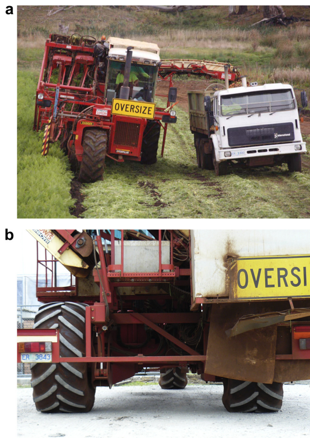
Fig. 1 – Front (a) and rear (b) views of tri-cycle carrot harvester showing wheel arrangements that are incompatible with CTF.
