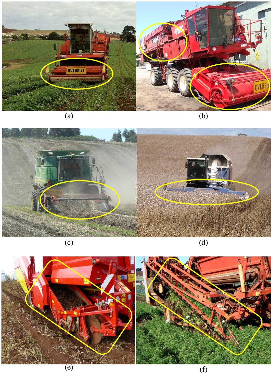
Figure 6-6. Crop collection components of existing harvesters that could possibly be adapted for use on a WS harvest tool carrier – (a) bean front, (b) pea front and viner, (c ) pyrethrum windrow front and thresher, (d) poppy front and mulcher, (e ) potato digger, (f) carrot top-lifter. (Source: J. McPhee)
