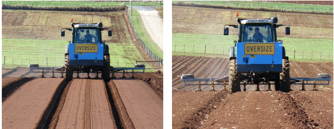
Figure 3-2. Bed surface condition formed by a smudge board bed former (left) compared to the wire roller (right).
