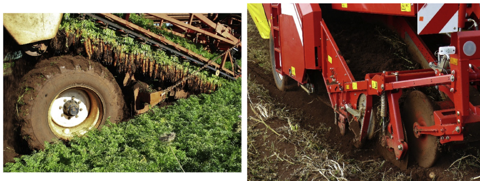
Fig. 4 – Current towed, bunker-style single-row carrot (left) and potato (right) harvesters are designed with one tyre tracking over the top of the dug row immediately after product removal, resulting in very high compaction risk.
