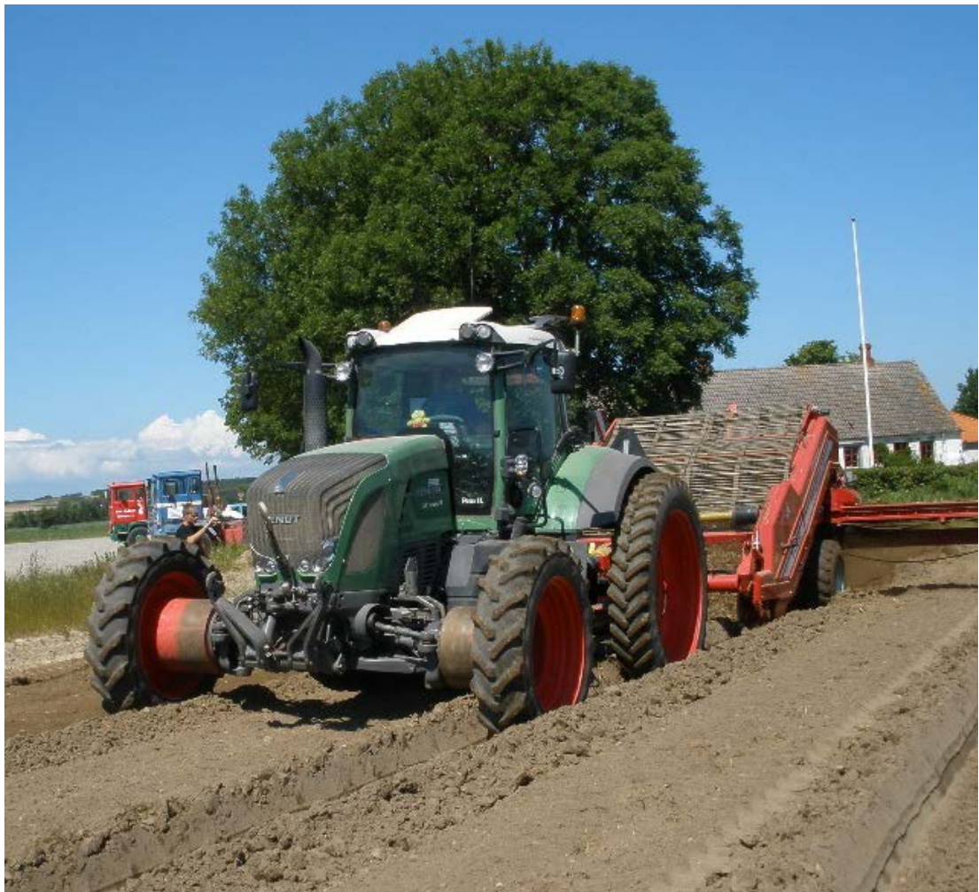
Figure 6-7. Conventional tractor with axles extended to 3.2 m to work in conjunction with the ASA-Lift WS9600. (Source: J. MCPhee)
