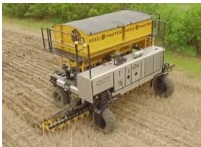
Figure 6-8. The DOT autonomous tool frame, which has potential to be used as a small wide span. (Source: DOT Farming Reimagined.
