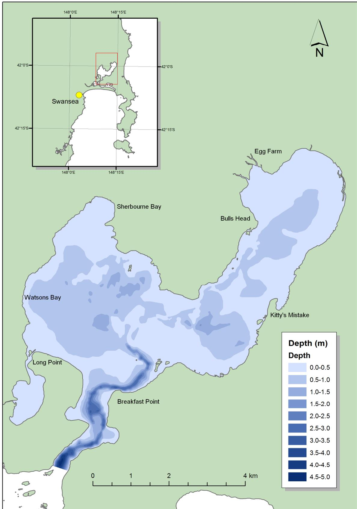
Figure 179. Map showing bathymetry of Moulting Lagoon interpolated from acoustic data.
