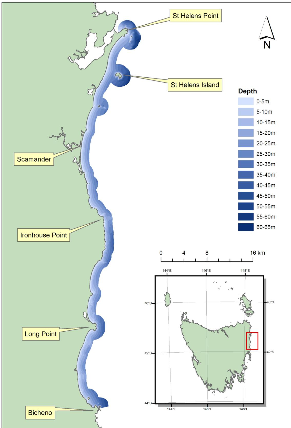
Figure 19. Map of bathymetry for Bicheno to St Helens based on interpolated acoustic data.
