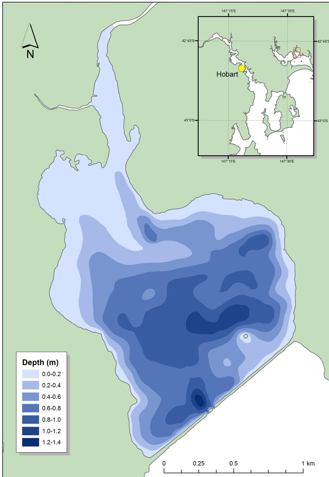
Figure 167. Map of bathymetry interpolated from acoustic data.
