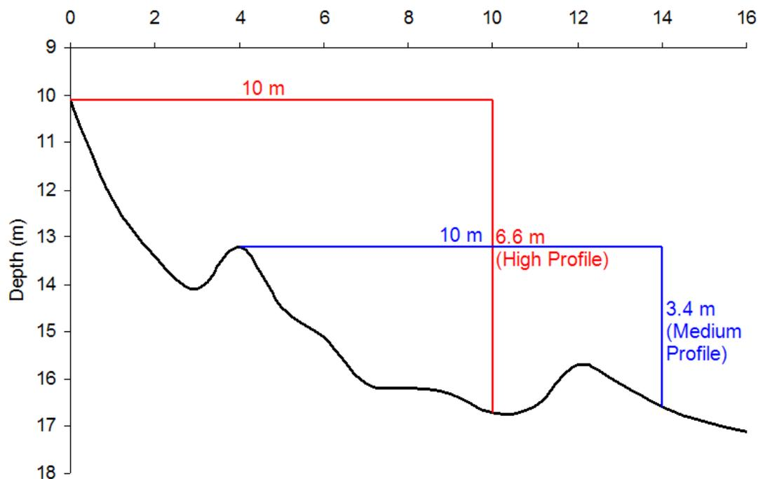
Figure showing two moving 10 metre windows (red and blue) used for calculating the reef profile across the sounder detected bottom (black line)
